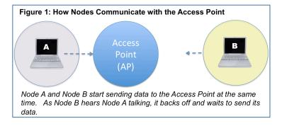
The mechanism used to determine the back off order is similar to right of way rules at a four-way stop. These rules of etiquette are followed to prevent a crash and allow each node to send its data unimpeded. Thus, 802.11 is designed with a set of courtesies such that if one node hears another node talking, it backs off, going silent as to reduce the chaos of multiple transmissions at the same time. This is true for every node in the network.
