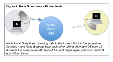
When a network with hidden nodes reaches capacity, it is usually due to circumstances such as this, where nodes with stronger signals steal the airwaves and crowd out nodes with weaker signals. If the nodes with the stronger signals continue to talk constantly, the weaker nodes can be locked out indefinitely, leaving certain users without access to the network.
